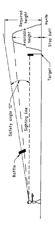
Figure 1 — Application of the safety angle (showing the use of a baffle)
